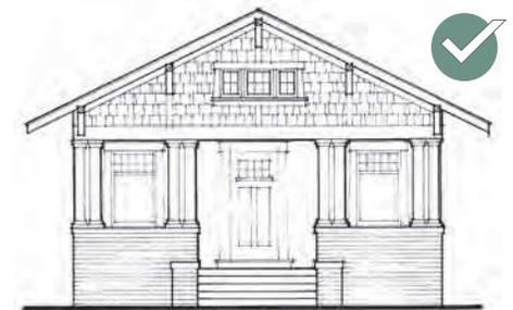
**Figure 8.9:** The top model illustrates a historic, vernacular house with an original porch that has been enclosed, which is an inappropriate treatment. The bottom model illustrates a replacement porch that has been designed similarly to the original porch, which is the preferred approach, when historic documentation is available.
