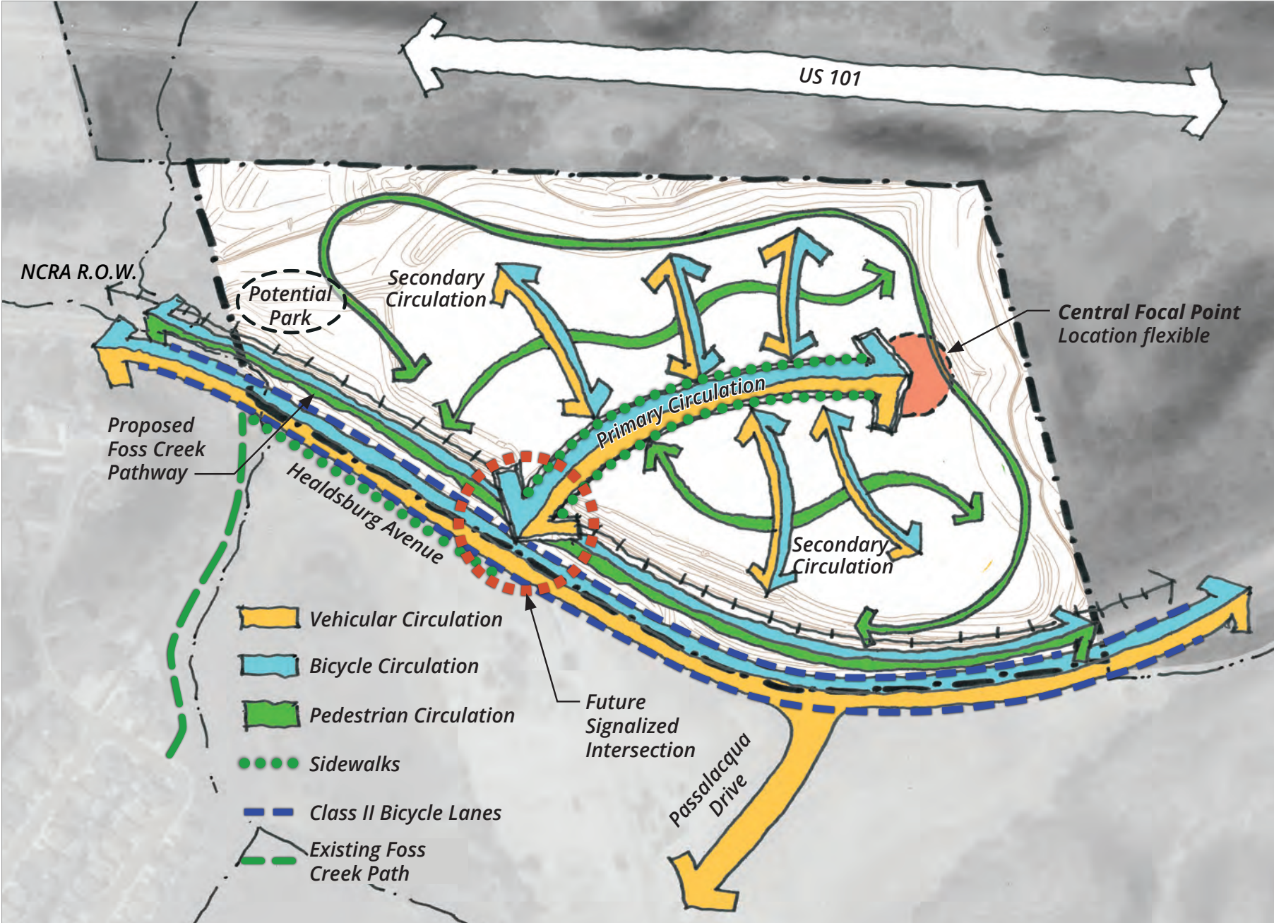
FIGURE 6-6: Access and Circulation
